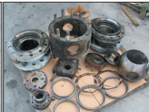
Complete Breakdown after Fire Test
