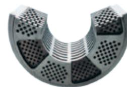
**VRT®**, Variable Resistance Trim, consists of a brazed stack of drilled plates which efficiently channel the flow through multiple turns in a tortuous path configuration. The design is primarily used in high-pressure drop liquid applications. VRT is typically packaged within standard Dresser Masoneilan globe and angle valve bodies.
