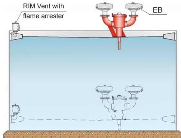
If resistance against endurance burning is not required the valves can alternatively be combined with PROTEGO® deflagration proof devices type PROTEGO® LH/AD. The applicable data sheets are available in volume 2 "Deflagration Flame Arresters, end-of-line and Vent Caps".
