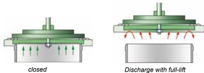
Figure 5b: Discharge with full-lift pallet and metal seal
