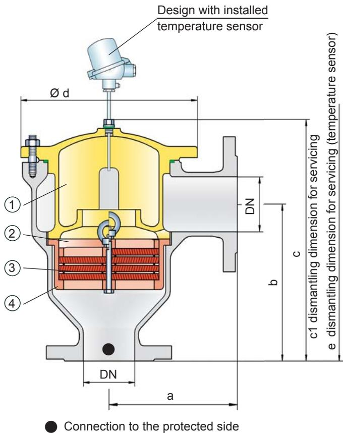
The standard design is approved at an operating temperature up to +60°C / 140°F and an absolute operating pressure up to 1.2 bar / 17.4 psi. Devices with special approvals can be obtained for higher pressures and higher temperatures upon request.
