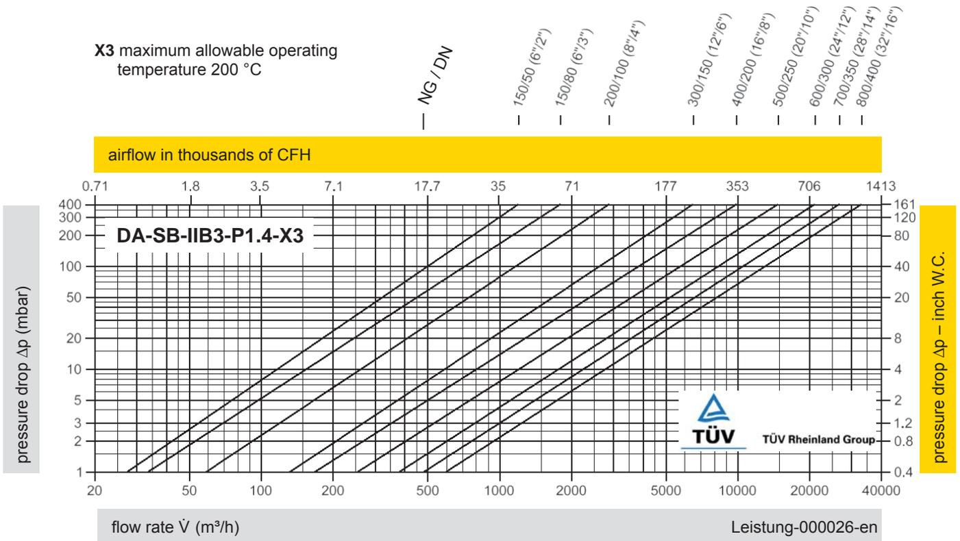
The flow capacity charts have been determined with a calibrated and TÜV certified flow capacity test rig.
