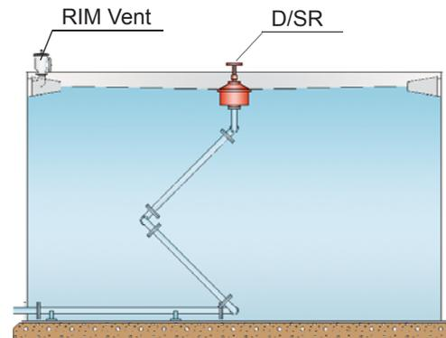
PROTEGO® roof drain valve type D/SR in combination with Floating roof drainage system PROTEGO® SE/CK
