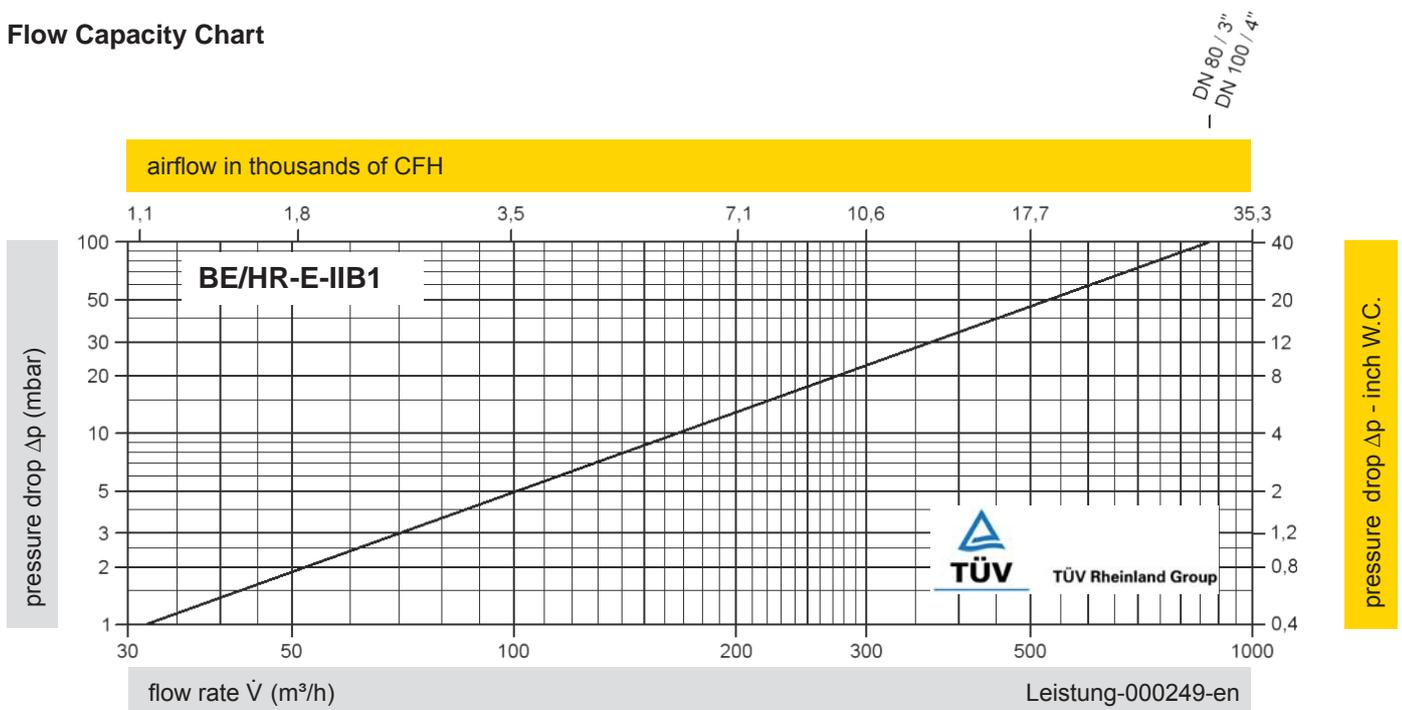
The flow capacity charts have been determined with a calibrated and TÜV certified flow capacity test rig. Volume flow  $\dot{V}$  in (m³/h) and CFH refer to the standard reference conditions of air ISO 6358 (20°C, 1bar). Conversion to other densities and temperatures refer to Vol. 1: "Technical Fundamentals".
