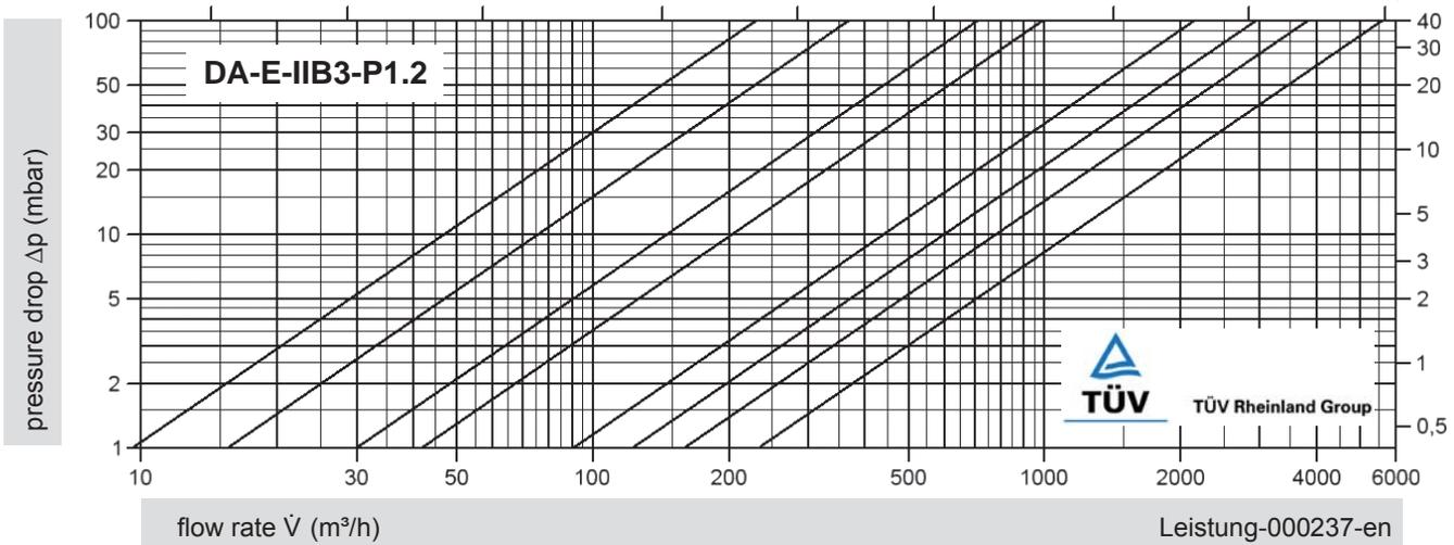
The flow capacity charts have been determined with a calibrated and TÜV certified flow capacity test rig.
