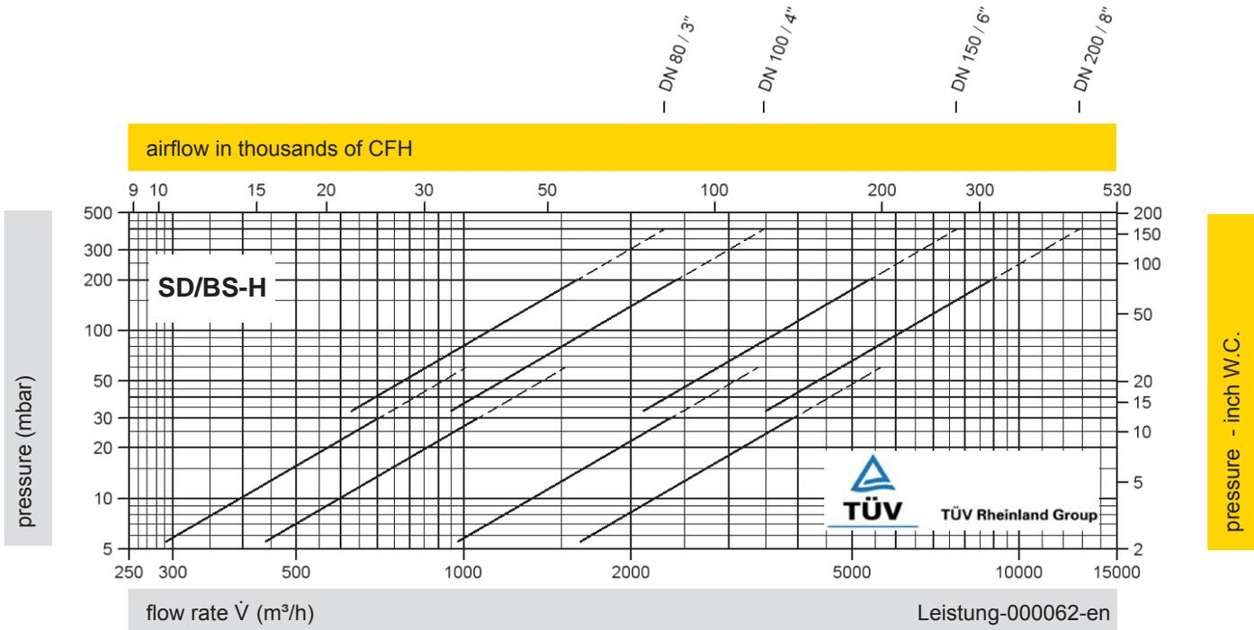
The flow capacity chart has been determined with a calibrated and TÜV certified flow capacity test rig. Volume flow  $\dot{V}$  in (m³/h) and CFH refer to the standard reference conditions of air ISO 6358 (20°C, 1bar). Conversion to other densities and temperatures refer to Vol. 1: "Technical Fundamentals".
