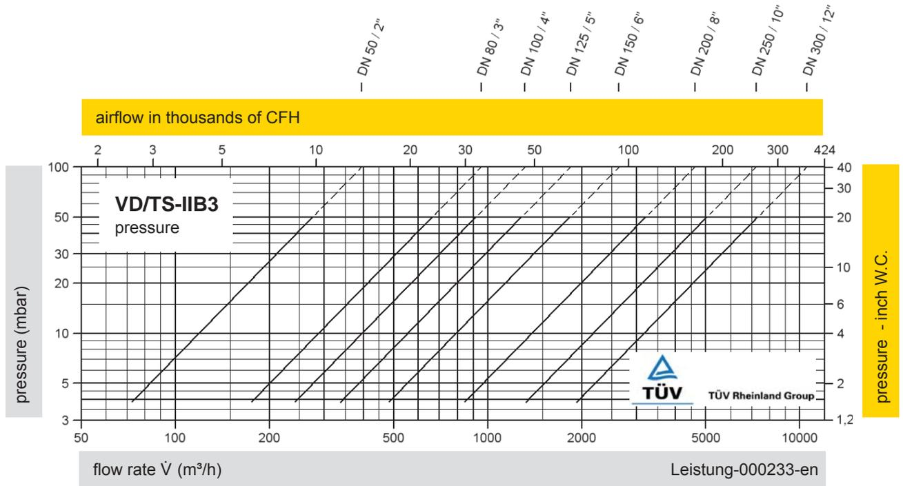
\* at set pressure of +22 to +50 mbar / +8.8 to +20 inch W.C. a volume flow reduction of 15% has to be made on the vacuum side
