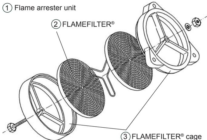
**Deflagration and short time burning proof end-of-line flame arresters** are equipped with a temperature sensor, which detects a stabilized flame on the flame arrester element. If a flame is detected, measures shall be taken to extinguish the flame and prevent endurance burning.
