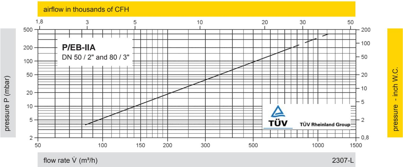
The flow capacity charts have been determined with a calibrated and TÜV certified flow capacity test rig. Volume flow  $\dot{V}$  in (m³/h) and CFH refer to the standard reference conditions of air ISO 6358 (20°C, 1bar). Conversion to other densities and temperatures refer to Vol. 1: "Technical Fundamentals".
