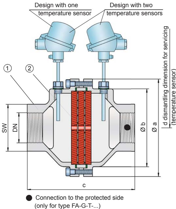
terminated by the operating data and parameters of the mixture flowing in the line (explosion group, pressure, temperature). The PROTEGO® FA-G series in-line deflagration flame arresters is available for explosion groups IIA, IIB3 and IIC (NEC groups D, C (MESG  $\geq 0.65$  mm) and B).
