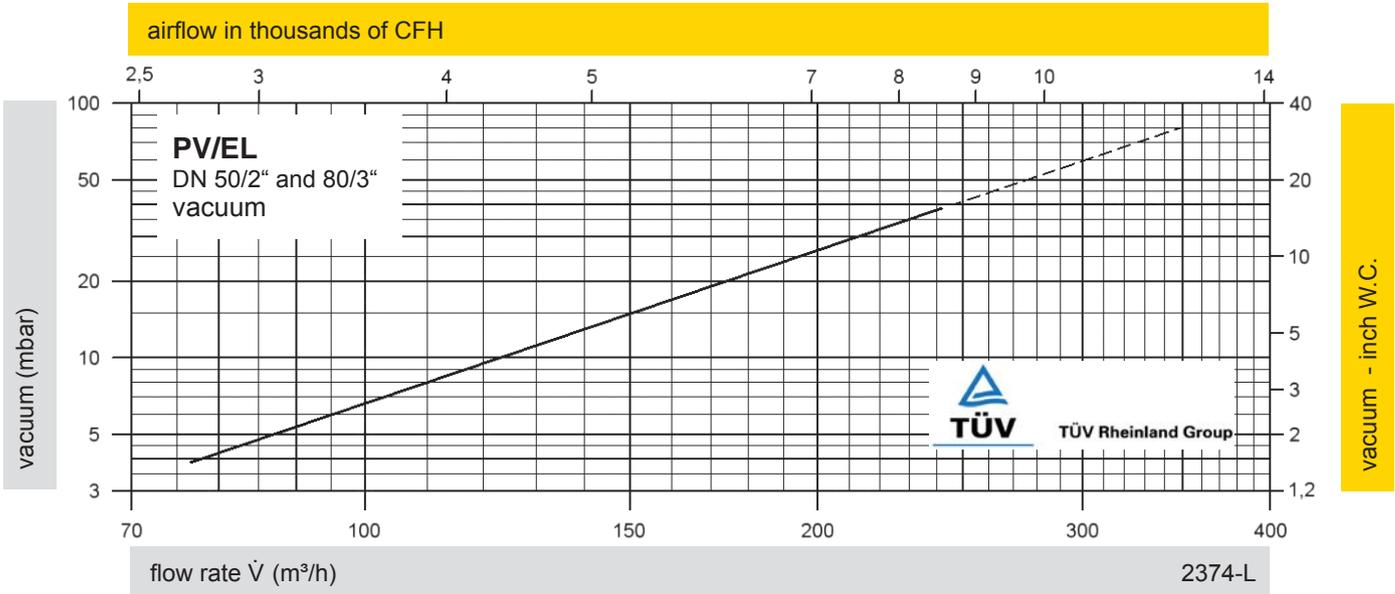
The flow capacity charts have been determined with a calibrated and TÜV certified flow capacity test rig. Volume flow  $\dot{V}$  in (m³/h) and CFH refer to the standard reference conditions of air ISO 6358 (20°C, 1bar). Conversion to other densities and temperatures refer to Vol. 1: "Technical Fundamentals".
