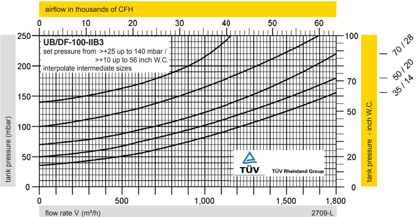
The flow capacity charts have been determined with a calibrated and TÜV certified flow capacity test rig. Volume flow  $\dot{V}$  in (m³/h) and CFH refer to the standard reference conditions of air ISO 6358 (20°C, 1bar). Conversion to other densities and temperatures refer to Vol. 1: "Technical Fundamentals".
