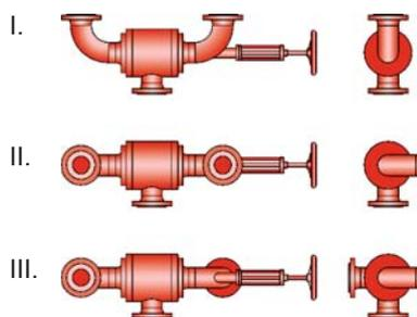
drag coefficient  $\zeta = 1,2$  for valve in center position
