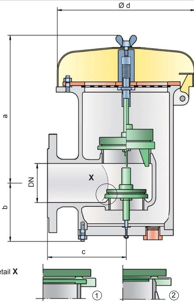
set just 10% below the maximum allowable working pressure or vacuum (MAWP or MAWV) of the tank and still safely vent the required mass flow. The opening characteristic is the same for pressure and vacuum relief.
