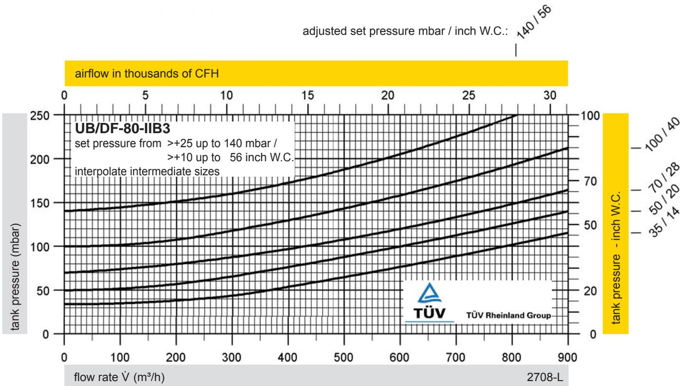
The flow capacity chart has been determined with a calibrated and TÜV certified flow capacity test rig.
