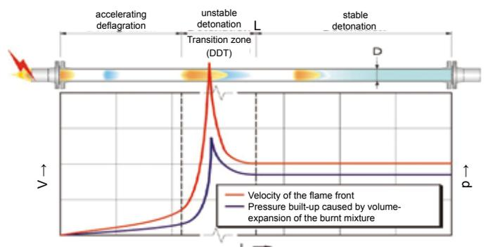
Figure 5: Deflagration – unstable detonation – stable detonation.
