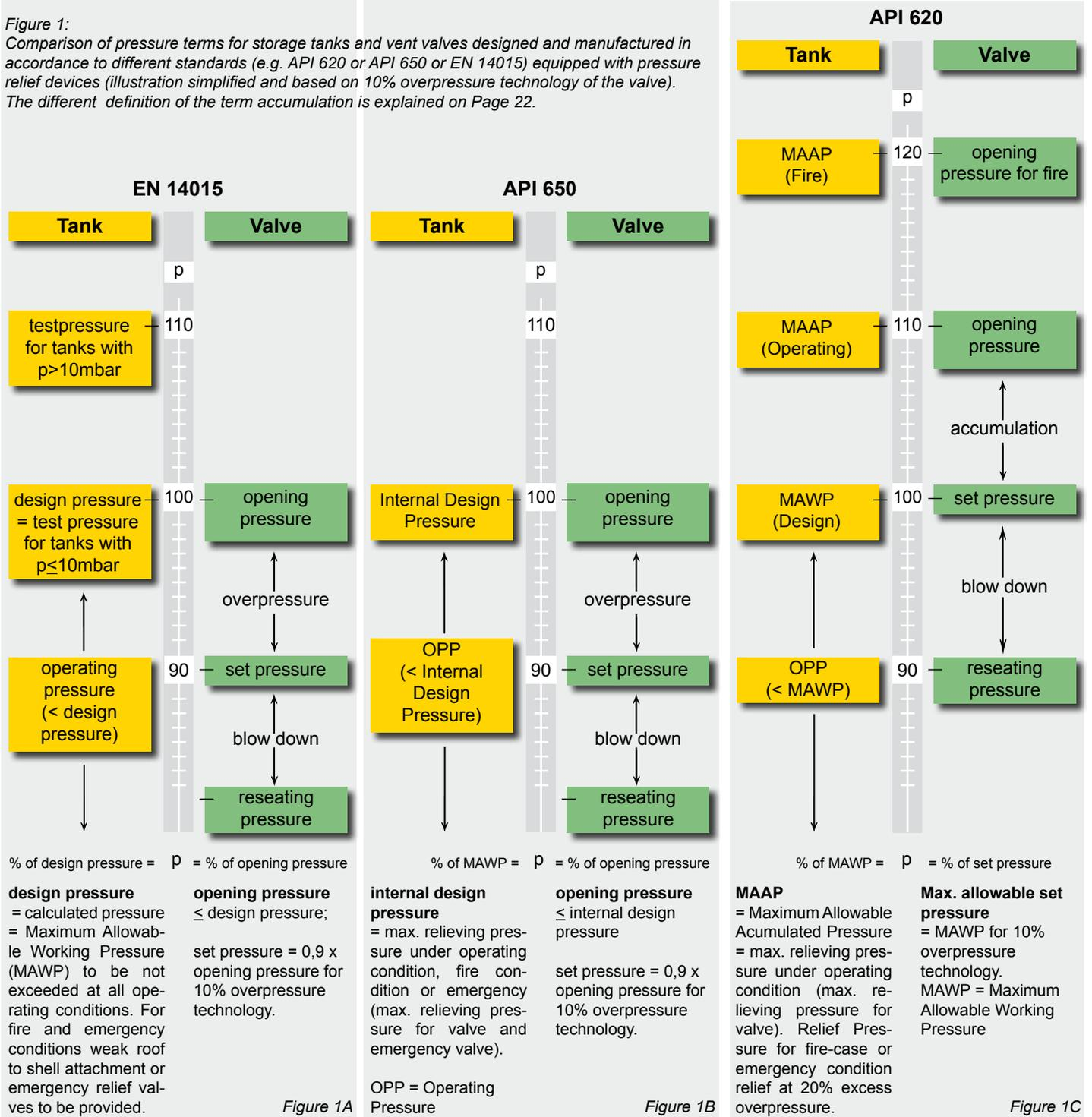
relieved. **Fig. 2** shows the procedure to determine the set pressure for valves with different overpressure characteristics by considering the specific tank design pressure. These examples are for end-of-line relief valves only without a back-pressure originated by e.g. connected pipe-away-line. If the tank is designed in accordance to EN 14015 or API 650 the opening pressure must not exceed the design pressure (=MAWP) of the tank (Fig. 2A). The set pressure
