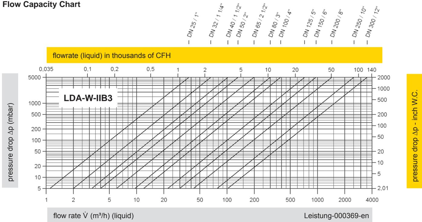
Conversion:  $\dot{V}_{liquid} = \dot{V}_{water} * \sqrt{\frac{\rho_{water}}{\rho_{liquid}}}$
