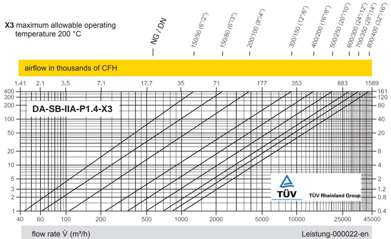
The flow capacity charts have been determined with a calibrated and TÜV certified flow capacity test rig. Volume flow  $\dot{V}$  in (m³/h) and CFH refer to the standard reference conditions of air ISO 6358 (20°C, 1bar). Conversion to other densities and temperatures refer to Vol. 1: "Technical Fundamentals".
