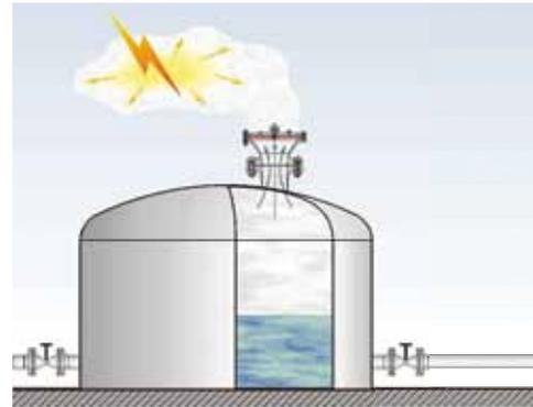
Figure 2: Atmospheric deflagration
