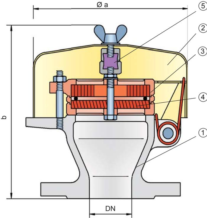
⑤ the spring loaded weather hood move into the open position. The PROTEGO® flame arrester unit consists of two FLAME-FILTER® discs (4), which are installed in a FLAMEFILTER® cage. The PROTEGO® BE/HK-E end-of-line deflagration flame arrester is available for alcohols and other substances with MESG  $\geq 0,85\text{mm}$ .
