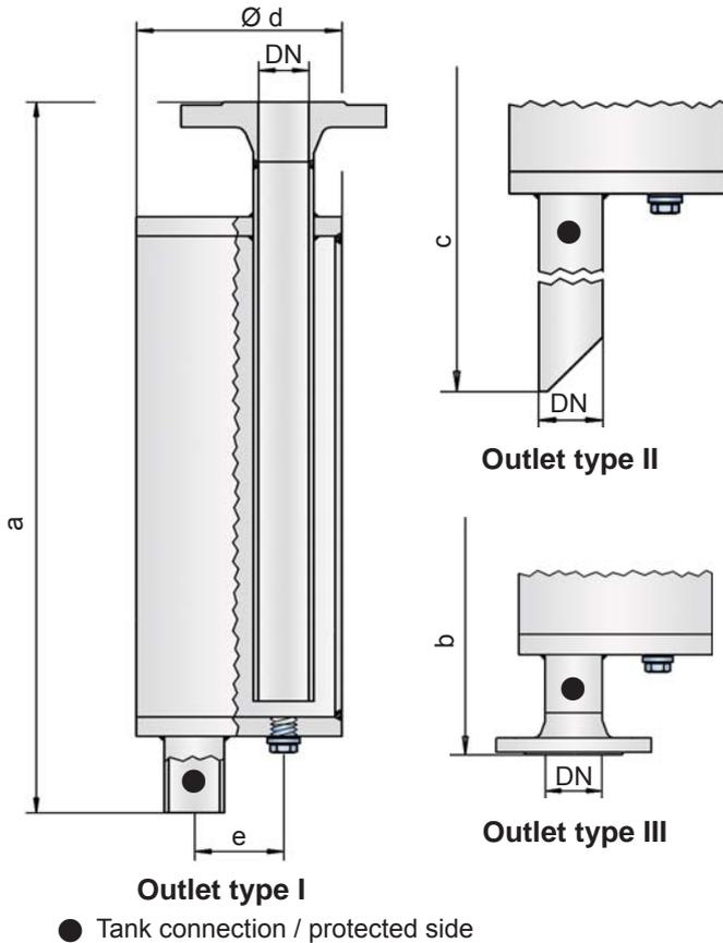
The device is installed inside the tank at the end of the line and prevents the combustion from being transferred into the tank if the explosive atmosphere ignites. The liquid detonation arresters function according to the siphon principle in which the liquid product serves as a liquid barrier to flame propagation.
