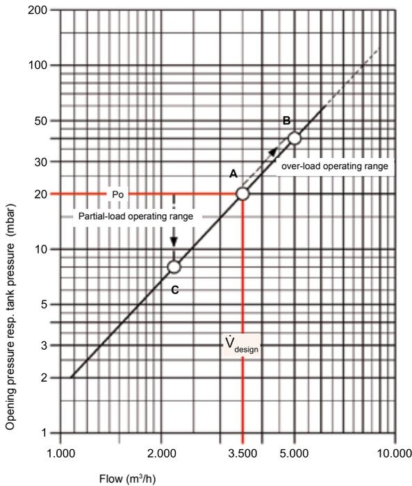
$$\text{set pressure} = \frac{\text{opening pressure resp. tank design pressure}}{1 + \frac{\text{overpressure \%}}{100\%}}$$
