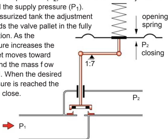
Should the tank pressure decrease the valve will open. If the plant is operated in a vacuum mode pressures down to -200 mbar / -80 inch W.C. relative pressure can be accommodated.
