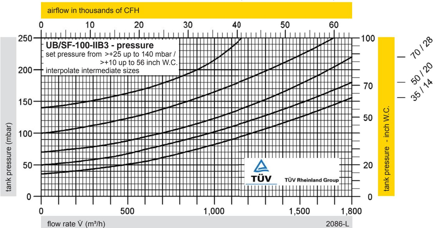
The flow capacity charts have been determined with a calibrated and TÜV certified flow capacity test rig. Volume flow  $\dot{V}$  in (m<sup>3</sup>/h) and CFH refer to the standard reference conditions of air ISO 6358 (20°C, 1bar). Conversion to other densities and temperatures refer to Vol. 1: "Technical Fundamentals".
