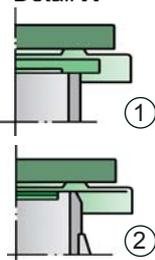
valve seats made of high quality stainless steel and with precisely lapped valve pallets (1) or with an air cushion seal (2) in conjunction with high quality FEP diaphragm. The valve pallets are also available with a PTFE seal to prevent the valve pallets from sticking when sticky products are used and to enable the use of corrosive fluids. After the excess pressure is discharged or the vacuum is compensated, the valve reseats and provides a tight seal.
