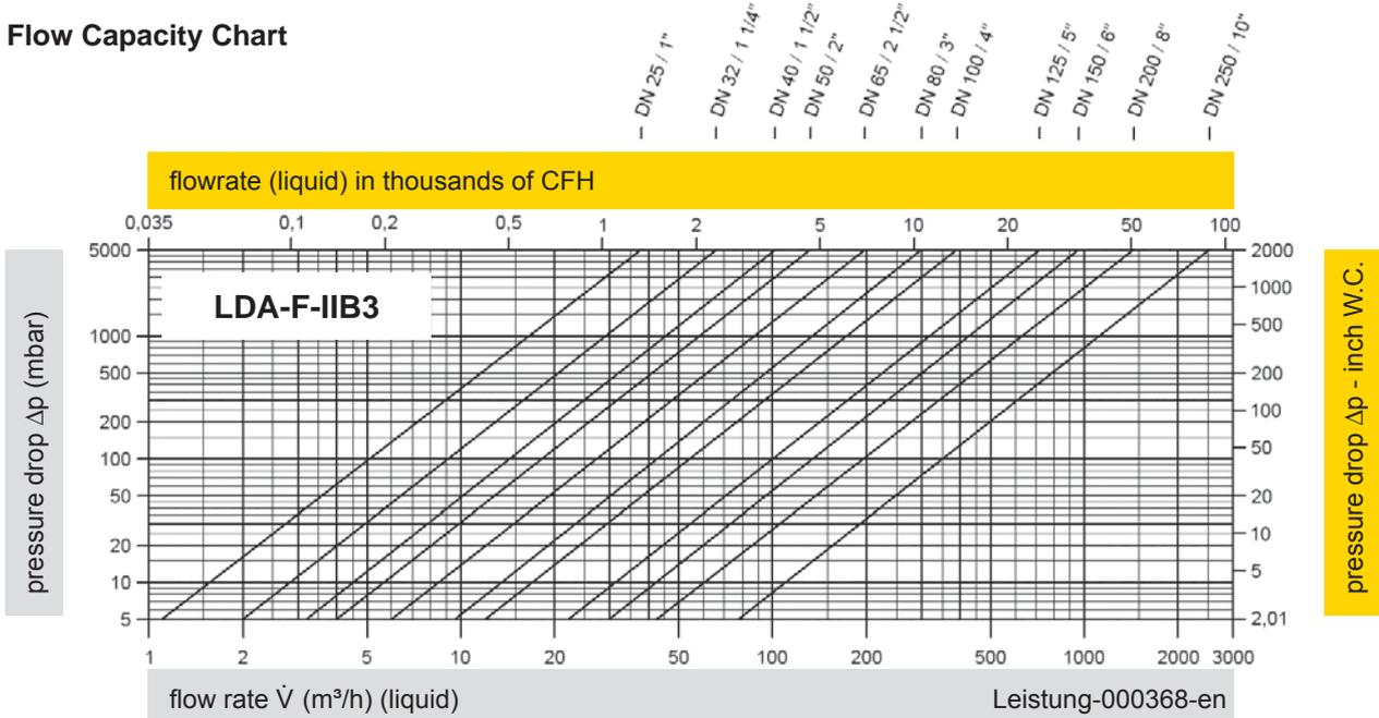
Conversion:  $\dot{V}_{liquid} = \dot{V}_{water} * \sqrt{\frac{\rho_{water}}{\rho_{liquid}}}$
