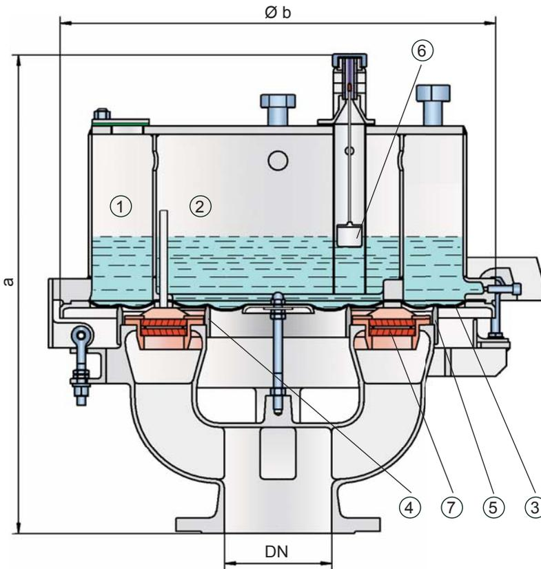
vacuum chamber, is reached the atmospheric pressure lifts the diaphragm (3) up off the inner and outer valve seat rings (4,5). Ambient air can now flow into the tank. The liquid column heights, which affect the set vacuum, can be checked by a floating level indicator (6).
