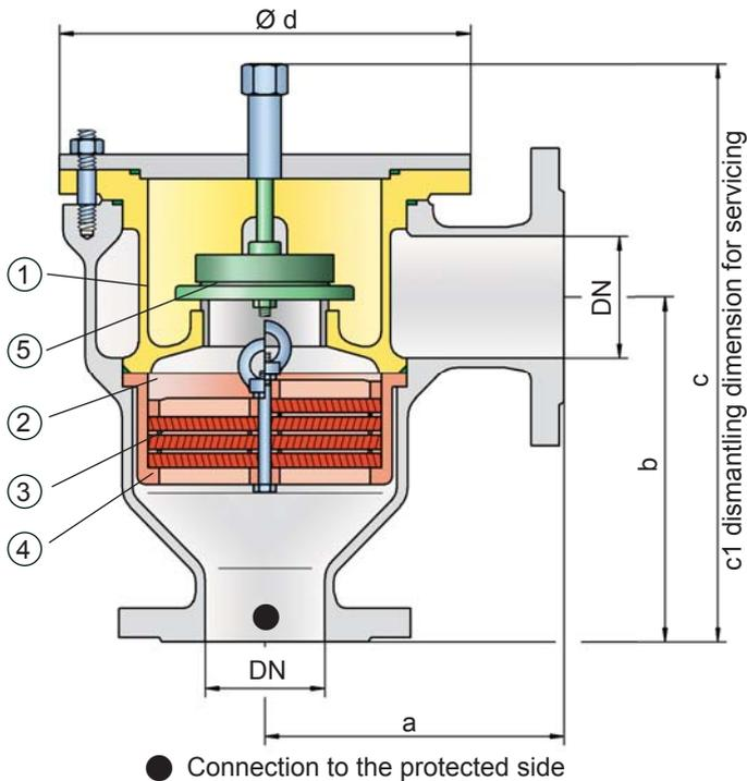
absorber, before the flame is extinguished in the narrow gaps of the FLAMEFILTER® (3). The flame suppression is guaranteed independent of the valve pallet position.
