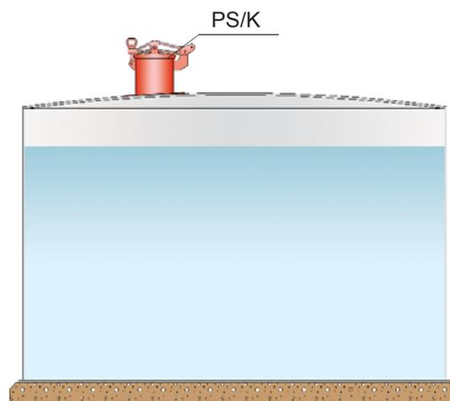
Gauge Hatches can be welded on tanks with floating roof.
