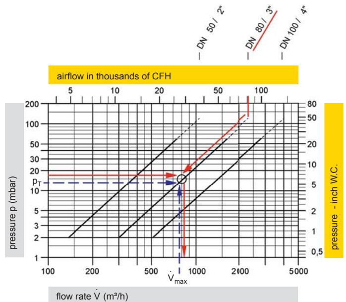
The set pressure of the valve (= valve starts to open) the maximum allowable pressure of the equipment minus the valves characteristic overpressure which is required for the valve to reach full lift.
