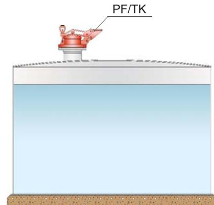
Gauge Hatches can be applied on tanks with floating roof.
