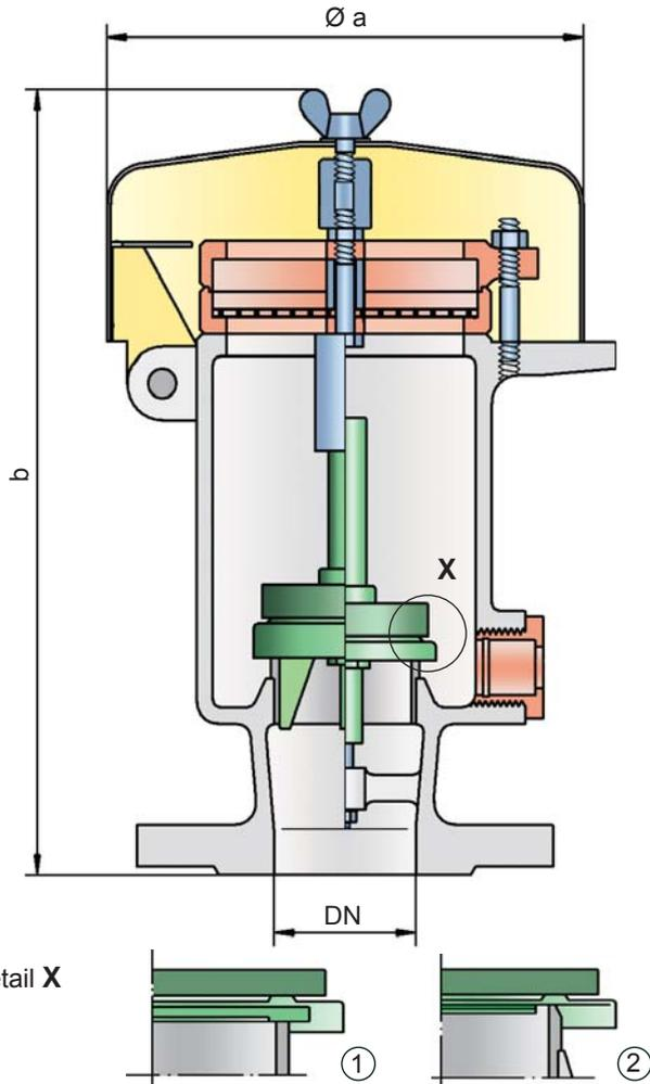
lowed PROTEGO® to develop a low pressure valve which has the same opening characteristic as a high pressure safety relief valve. This “full lift type” technology allows the valve to be set just 10% below the maximum allowable working pressure of the tank and still safely vent the required mass flow.
