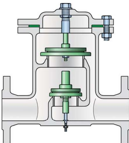
**PROTEGO® pressure relief valves** provide protection against unallowable high pressure and prevent emission losses almost up to set pressure.
