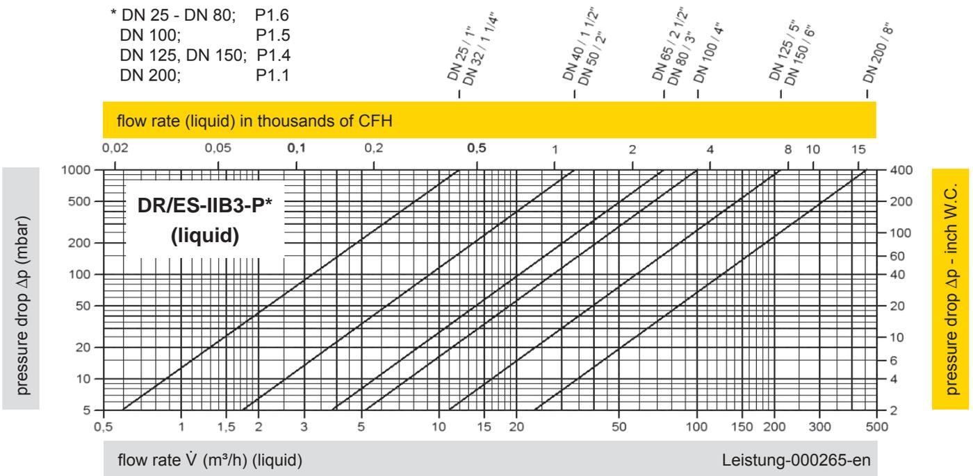
$$\text{Conversion: } \dot{V}_{\text{liquid}} = \dot{V}_{\text{water}} * \sqrt{\frac{\rho_{\text{water}}}{\rho_{\text{liquid}}}}$$
