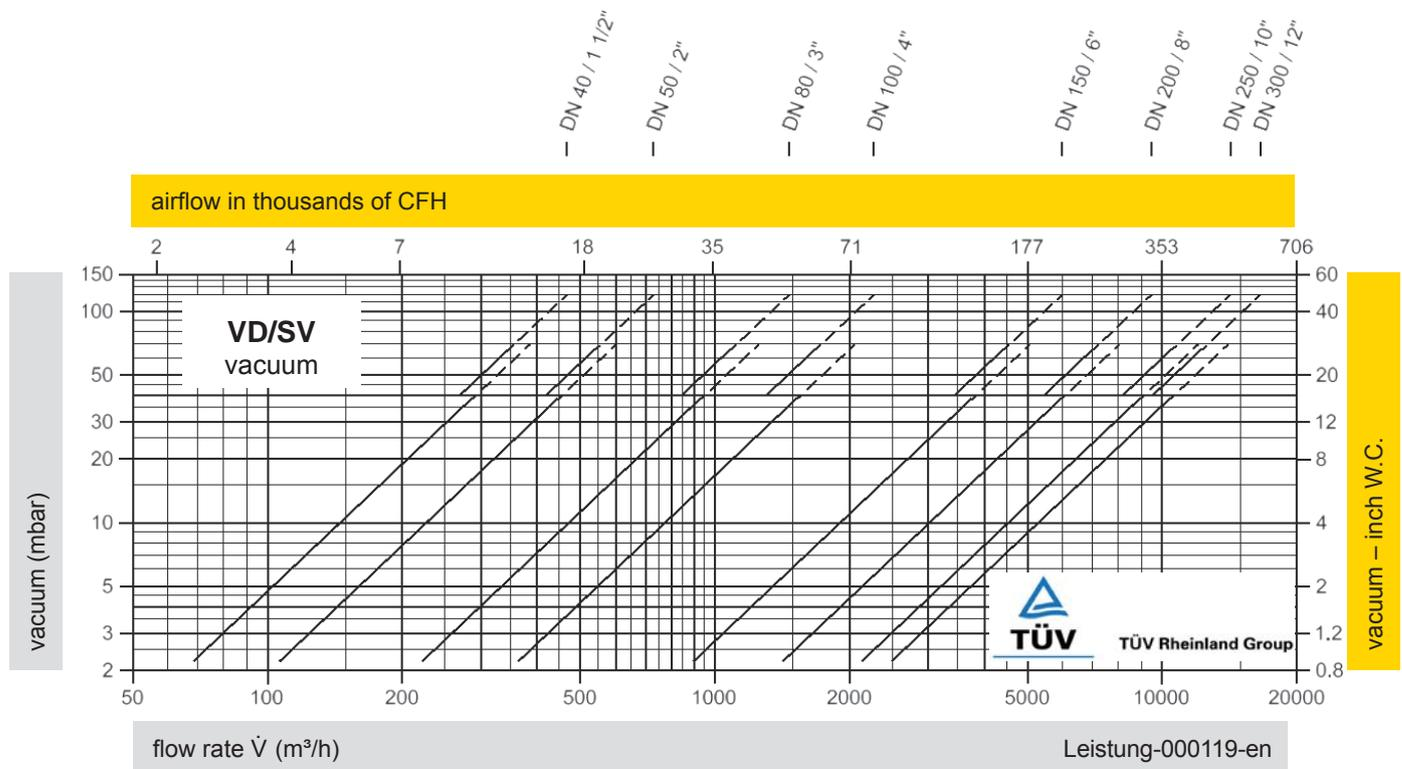
The flow capacity charts have been determined with a calibrated and TÜV certified flow capacity test rig. Volume flow  $\dot{V}$  in (m³/h) and CFH refer to the standard reference conditions of air ISO 6358 (20°C, 1bar). Conversion to other densities and temperatures refer to Vol. 1: "Technical Fundamentals".
