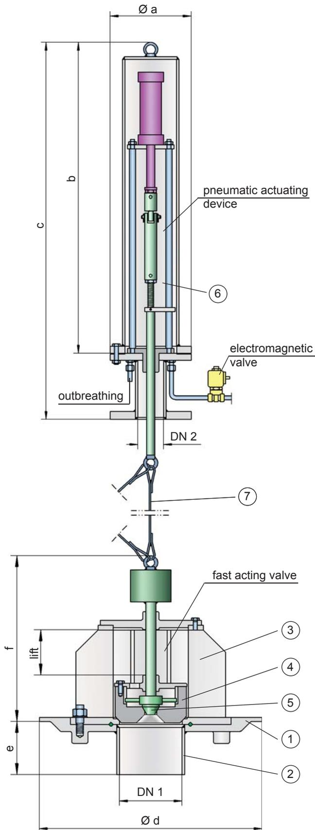
If fast acting valve is open, drag coefficient amounts to 1,5
