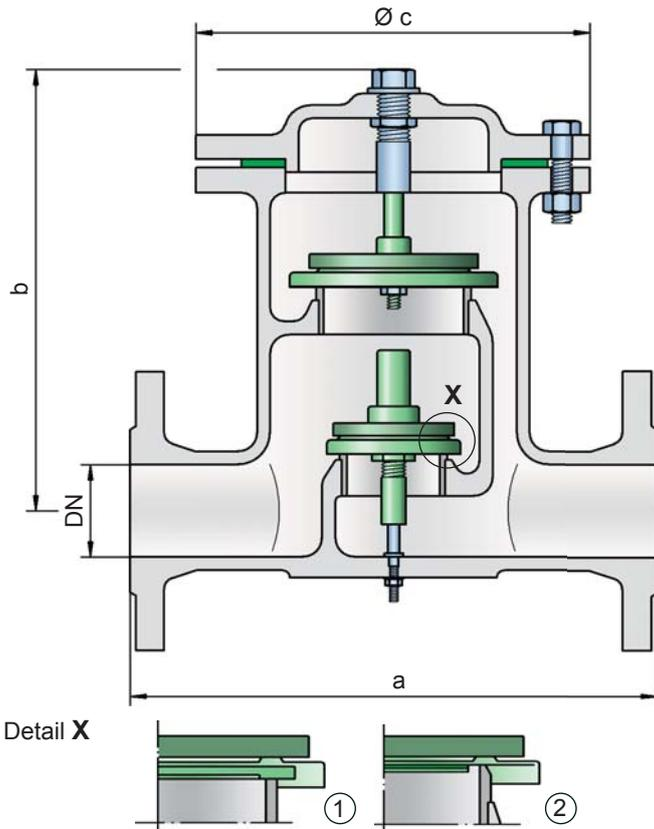
Tank connection depends upon flow capacity, set pressure and set vacuum for in- and outbreathing
