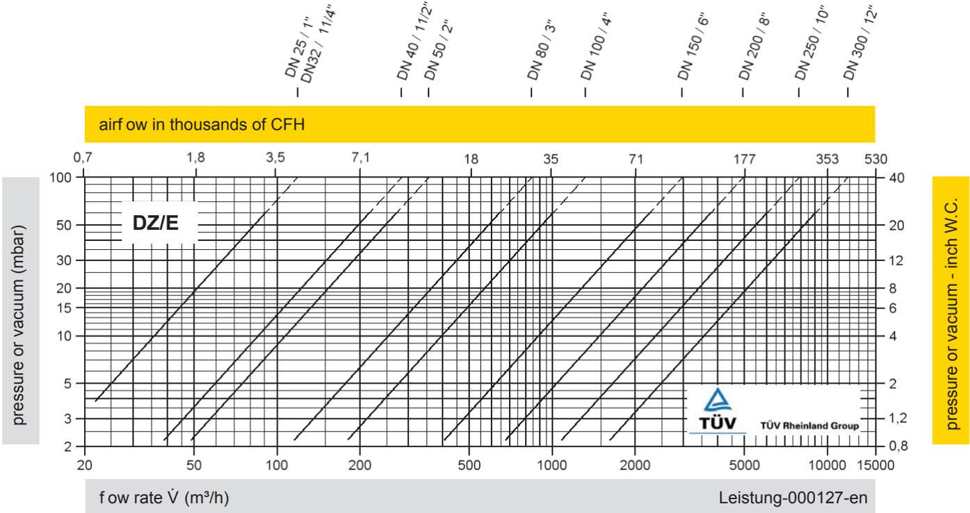
The flow capacity chart has been determined with a calibrated and TÜV certified flow capacity test rig. Volume flow  $\dot{V}$  in (m³/h) and CFH refer to the standard reference conditions of air ISO 6358 (20°C, 1bar). Conversion to other densities and temperatures refer to Technical Fundamentals.
