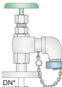
\* Position of drilling holes on flange connection as well as thickness upon request for size DN15 / ½", DN20 / ¾", DN25 / 1", DN32 / 1¼", DN40 / 1½" and pressure nominal PN25/40 resp. PN100 available.
