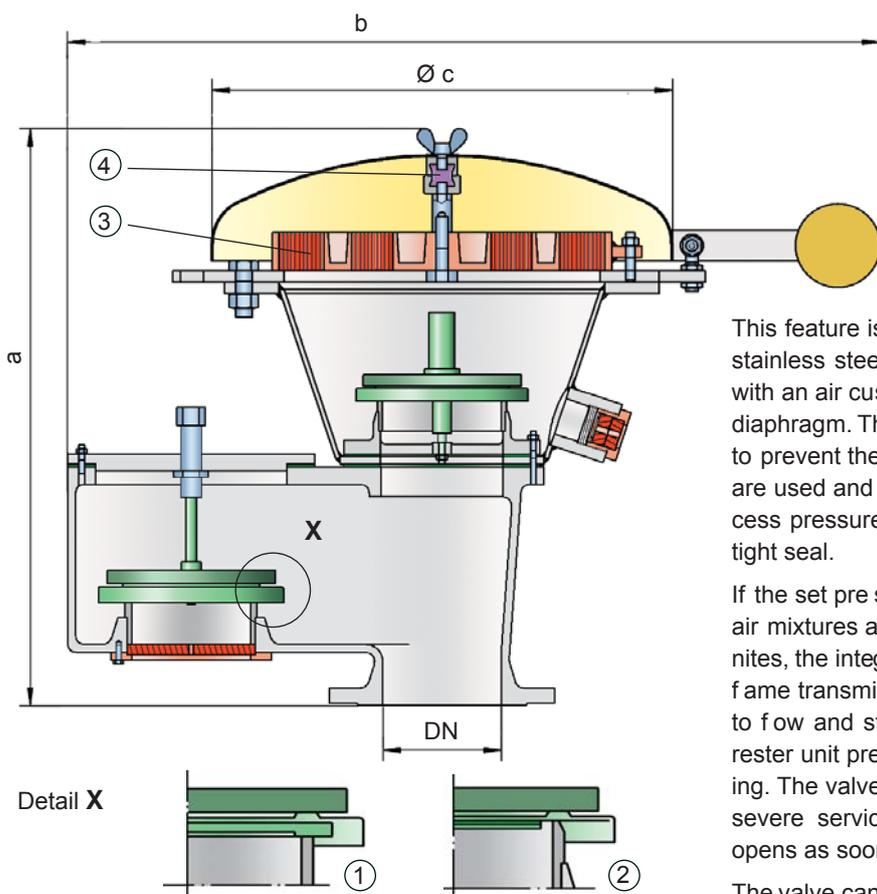
allowable working vacuum (MA WV) of the tank. After years of development, this typical opening characteristic of a safety relief valve is now also available for the low pressure range.
