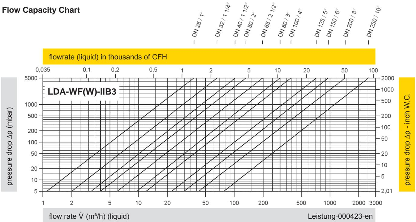
Conversion:  $\dot{V}_{liquid} = \dot{V}_{water} * \sqrt{\frac{\rho_{water}}{\rho_{liquid}}}$
