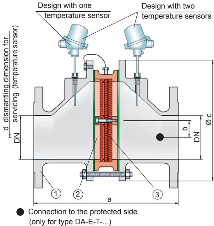
can be selected. The PROTEGO® DA-E series of flame arresters is available for explosion groups IIA to IIB3 (NEC Group D to C MESH  $\geq 0.65$  mm).
