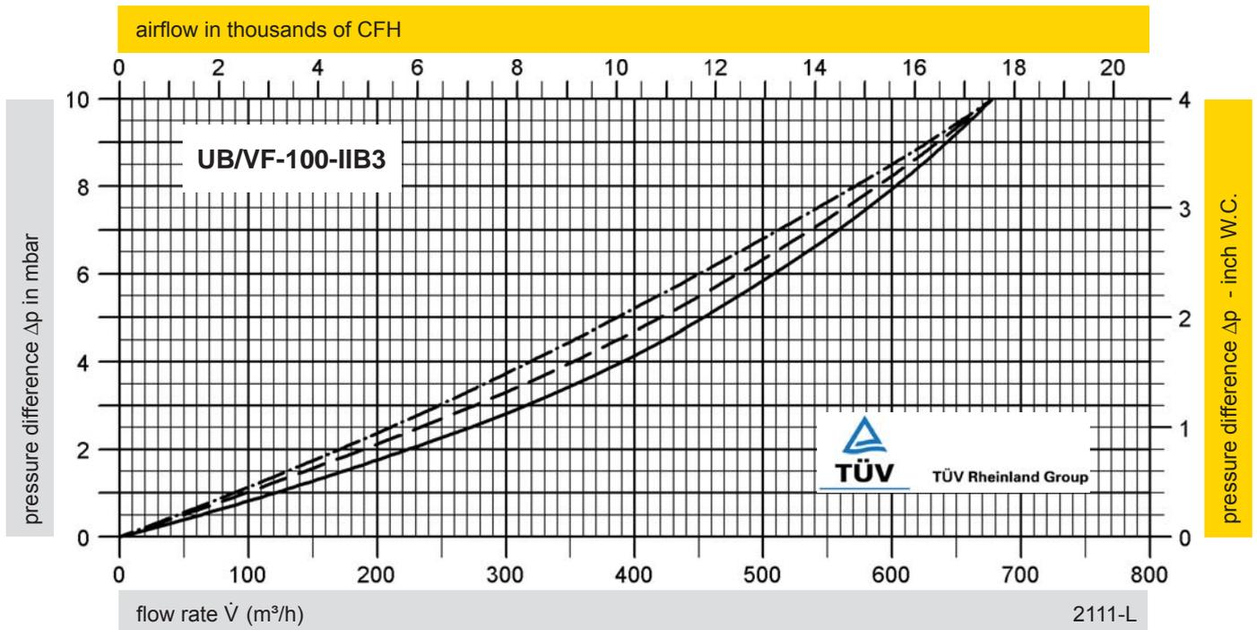
pressure difference = max. allowable tank design vacuum - valve set vacuum
