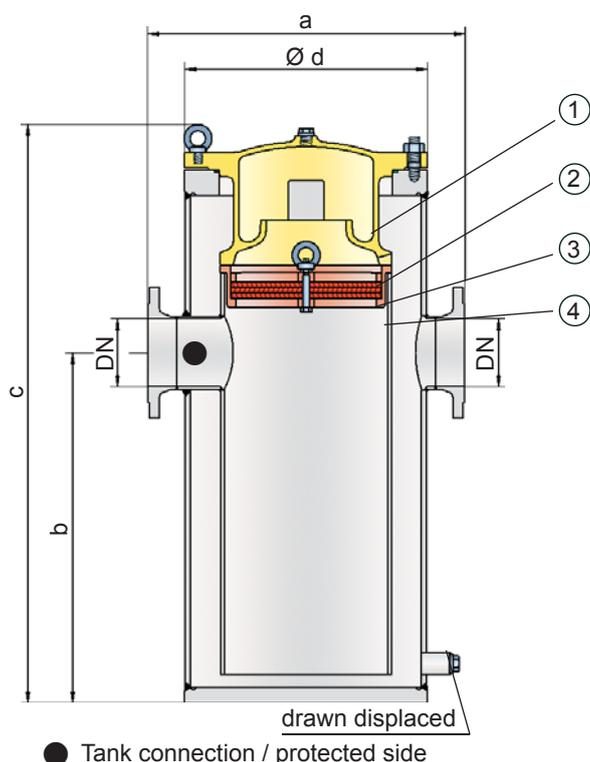
sphere is ignited, the device prevents the combustion from traveling into the tank. The PROTEGO® LDA-WF(W) series of liquid detonation flame arresters combines the classic PROTEGO® flame arrester design with the siphon principle in which the liquid product serves as a barrier to flame propagation.
