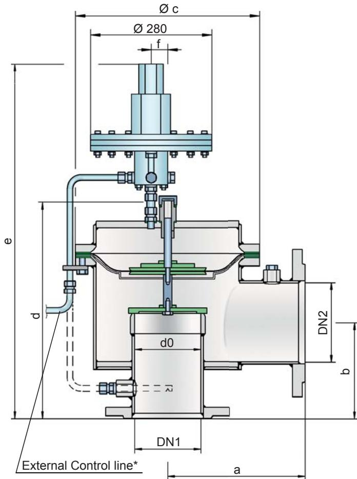
The main valve is controlled by a pilot valve. The latter in turn is controlled by the tank pressure. A small amount fluid stored in the tank released into the atmosphere by the pilot when the valve opens. The set-to-operate pressure is adjusted on the pilot valve by increasing or decreasing (as appropriate) the tension of a spring.
