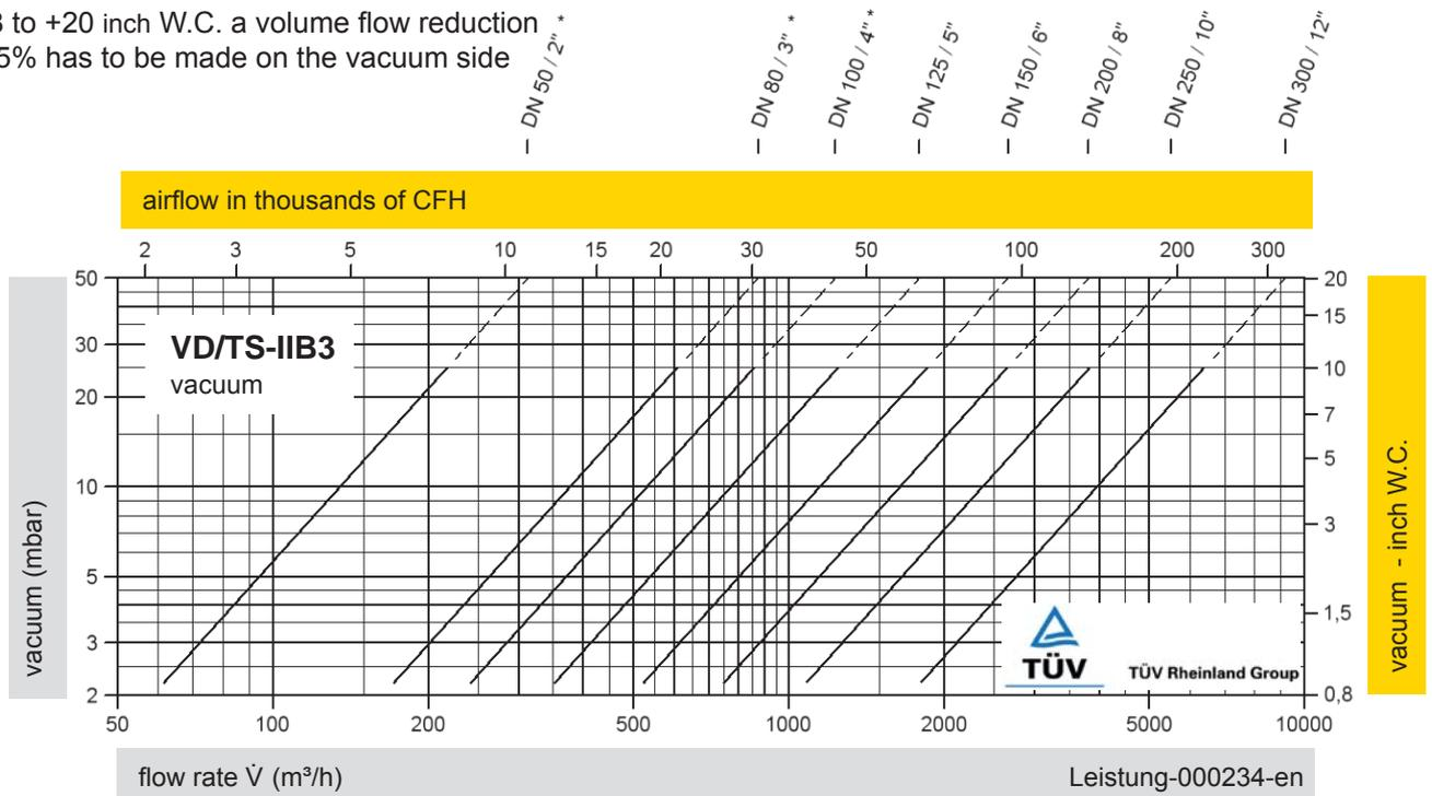
The flow capacity chart has been determined with a calibrated and TÜV certified flow capacity test rig. Volume flow  $\dot{V}$  in (m<sup>3</sup>/h) and CFH refer to the standard reference conditions of air ISO 6358 (20°C, 1bar). Conversion to other densities and temperatures refer to Vol. 1: "Technical Fundamentals".
