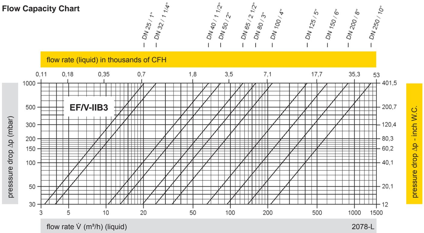
$$\text{Conversion: } \dot{V}_{\text{liquid}} = \dot{V}_{\text{water}} * \sqrt{\frac{\rho_{\text{water}}}{\rho_{\text{liquid}}}}$$
