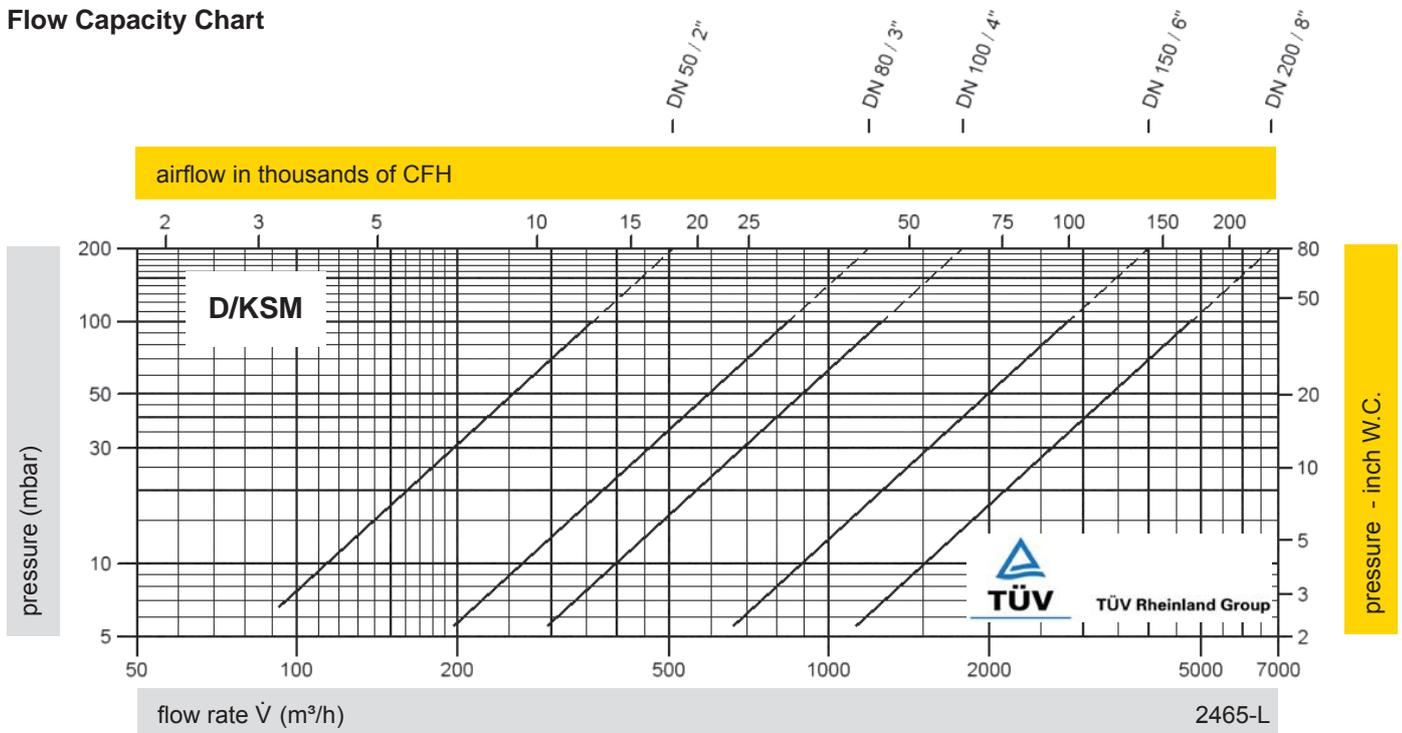
The flow capacity chart has been determined with a calibrated and TÜV certified flow capacity test rig. Volume flow  $\dot{V}$  in (m<sup>3</sup>/h) and CFH refer to the standard reference conditions of air ISO 6358 (20°C, 1bar). Conversion to other densities and temperatures refer to Vol. 1: "Technical Fundamentals".
