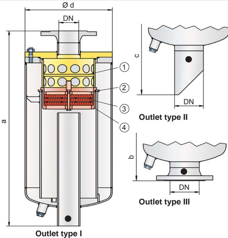
conditions of use. The device is installed inside the container at the end of the line and prevents the combustion from being transferred into the tank if the explosive atmosphere ignites. The PROTEGO® LDA-F series of liquid detonation arresters combines the classic PROTEGO® flame arrester design with the siphon principle in which the liquid product serves as a barrier to flame propagation.
