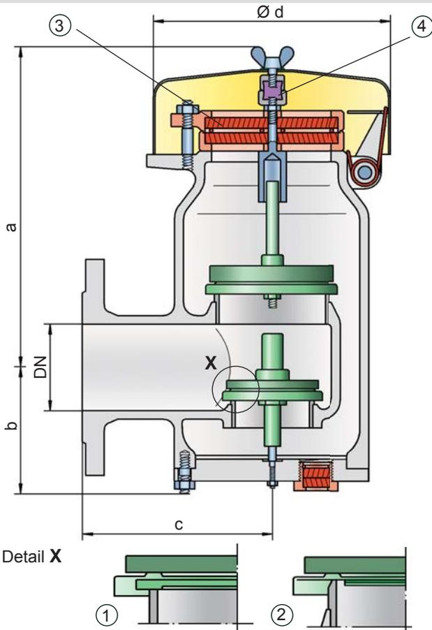
allowable working vacuum (MAWV) of the tank. After years of development, this typical opening characteristic of a safety relief valve is now also available for the low pressure range.
