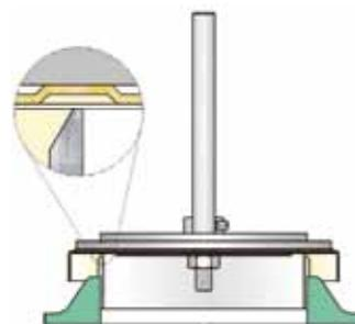
Figure 4: PROTEGO® full-lift pallet with air cushion seal
