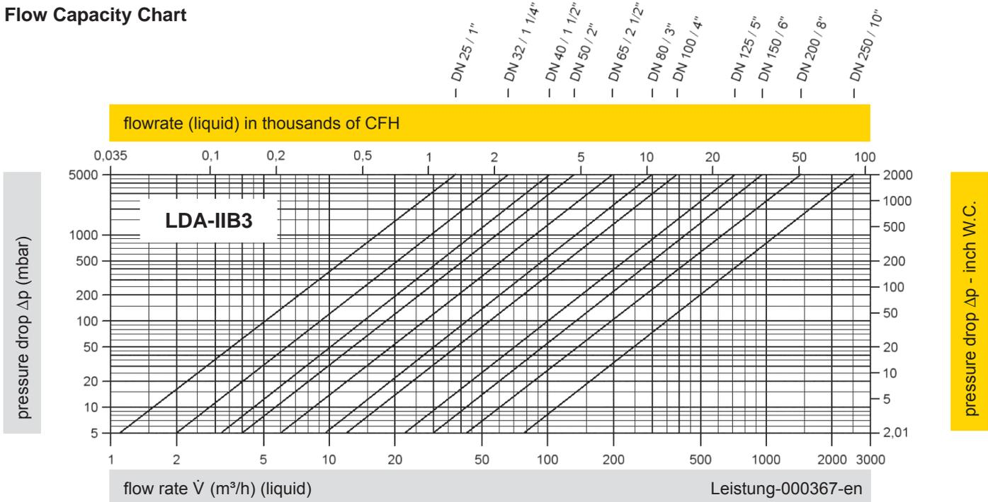
$$\text{Conversion: } \dot{V}_{\text{liquid}} = \dot{V}_{\text{water}} * \sqrt{\frac{\rho_{\text{water}}}{\rho_{\text{liquid}}}}$$
