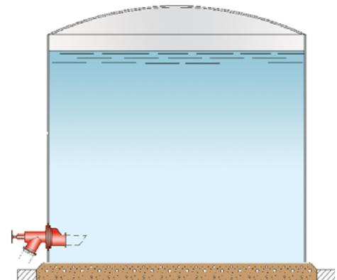
PROTEGO® SI/FA with internal connection nozzle
