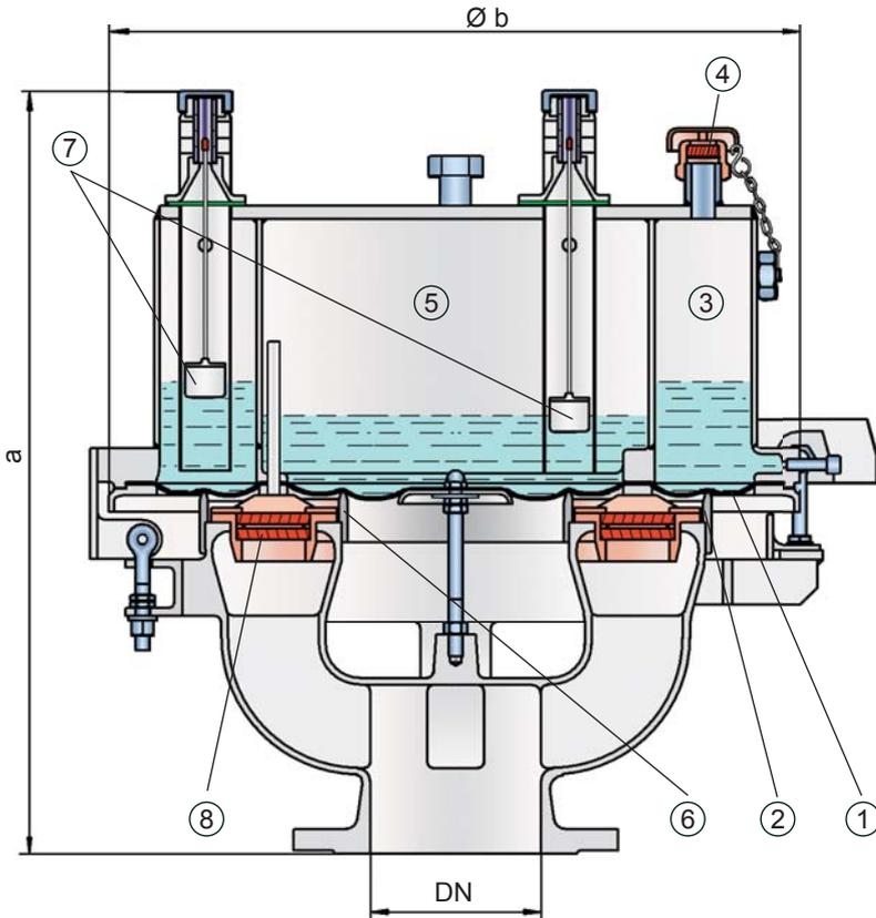
The set pressure is adjusted with a freeze resistant water-glycol mixture, which assures safe operation under extreme cold weather conditions. The PROTEGO® UB/SF valve is available for substances of explosion group IIB3 (NEC group C MESH  $\geq 0.65$  mm).
