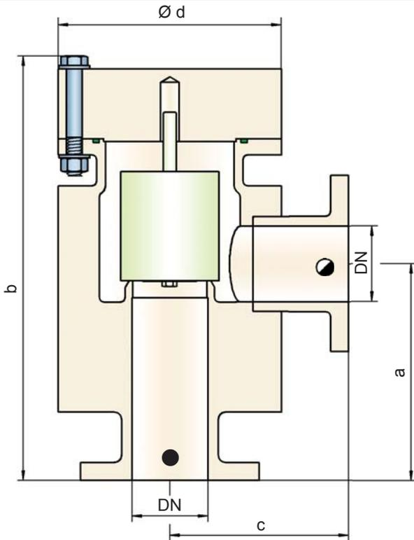
● = Tank connection for pressure relief function
