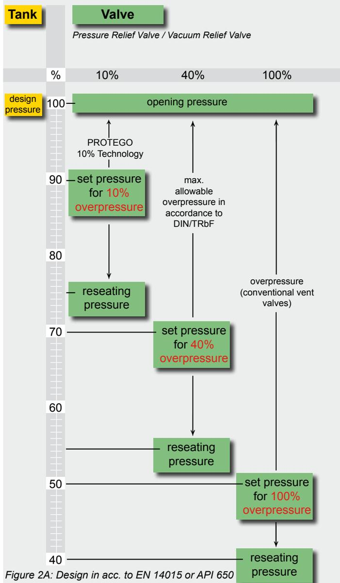
Figure 2A: Design in acc. to EN 14015 or API 650
