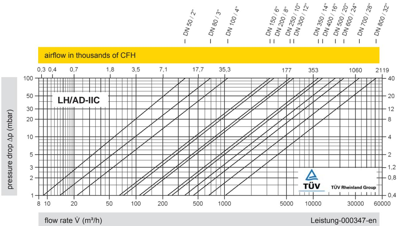
The flow capacity charts have been determined with a calibrated and TÜV certified flow capacity test rig. Volume flow  $\dot{V}$  in (m³/h) and CFH refer to the standard reference conditions of air ISO 6358 (20°C, 1bar). Conversion to other densities and temperatures refer to Vol. 1: "Technical Fundamentals".
