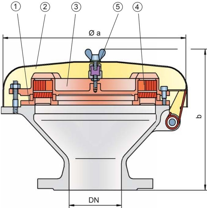
The PROTEGO® BE/HR-E end-of-line deflagration flame arrester is available for alcohols and other substances with a MESG  $\geq 0,85$  mm.
