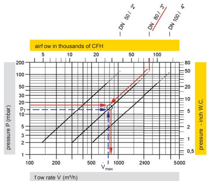
The required set pressure (= start of opening) will be the opening pressure (valve fully open) minus the characteristic overpressure.
