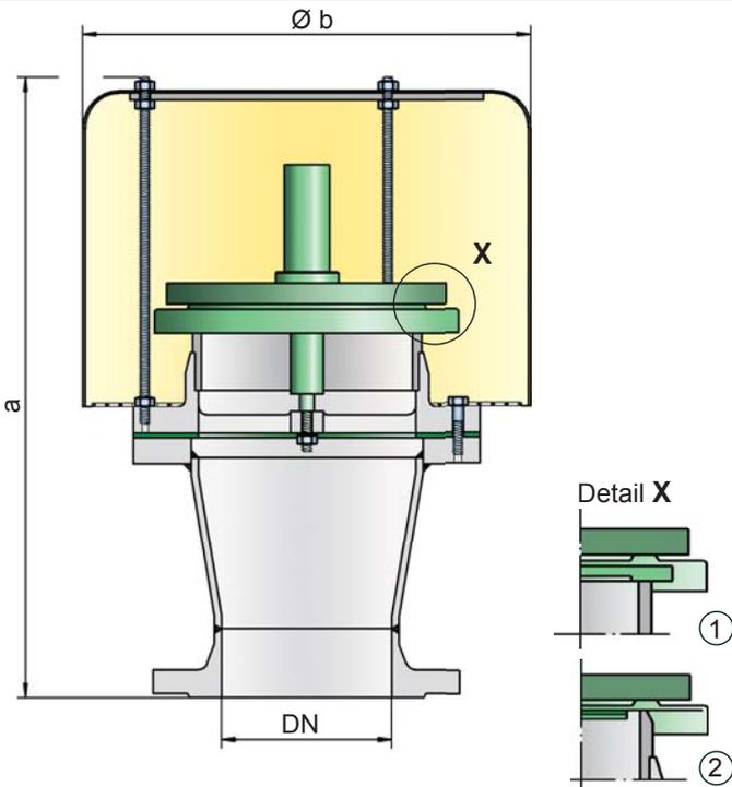
the same opening characteristic as a high pressure safety relief valve. This “full lift type” technology allows the valve to be set just 10% below the maximum allowable working pressure of the tank and still safely vent the required mass flow.
