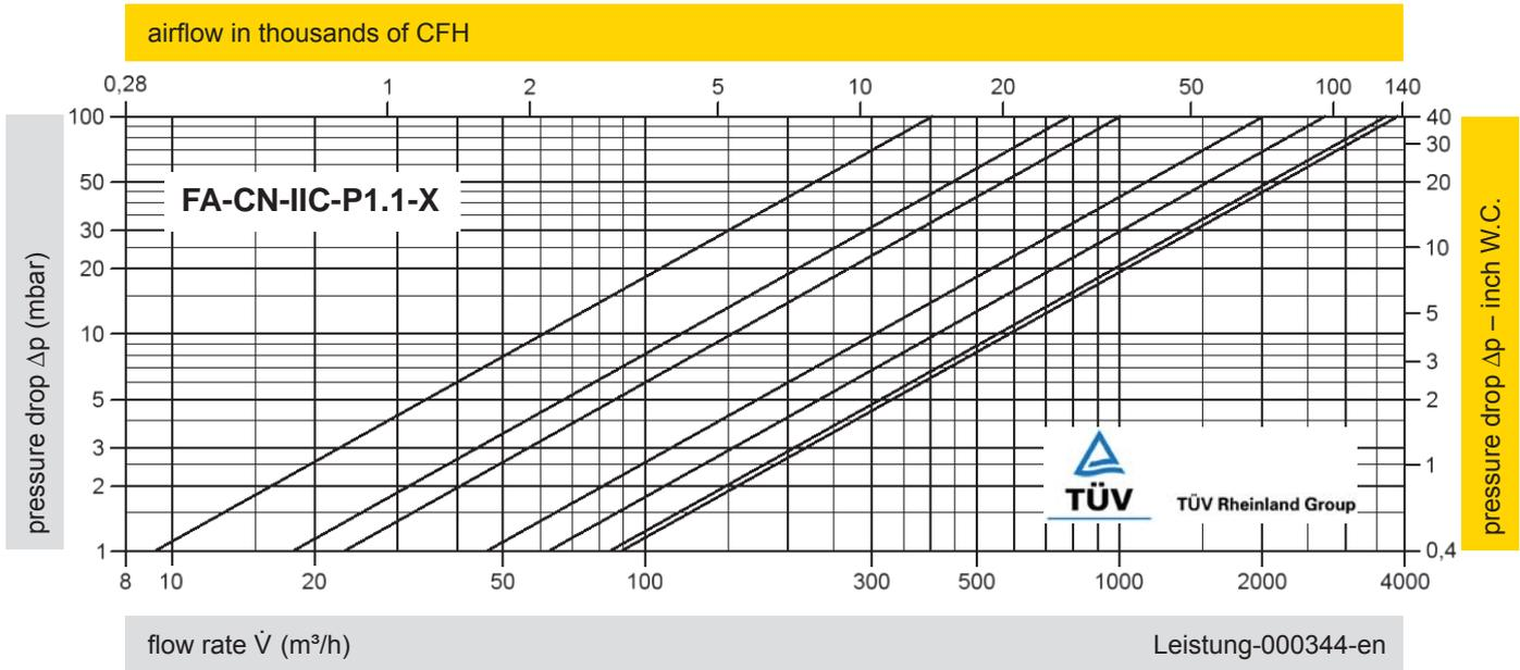
The flow capacity chart has been determined with a calibrated and TÜV certified flow capacity test rig.
