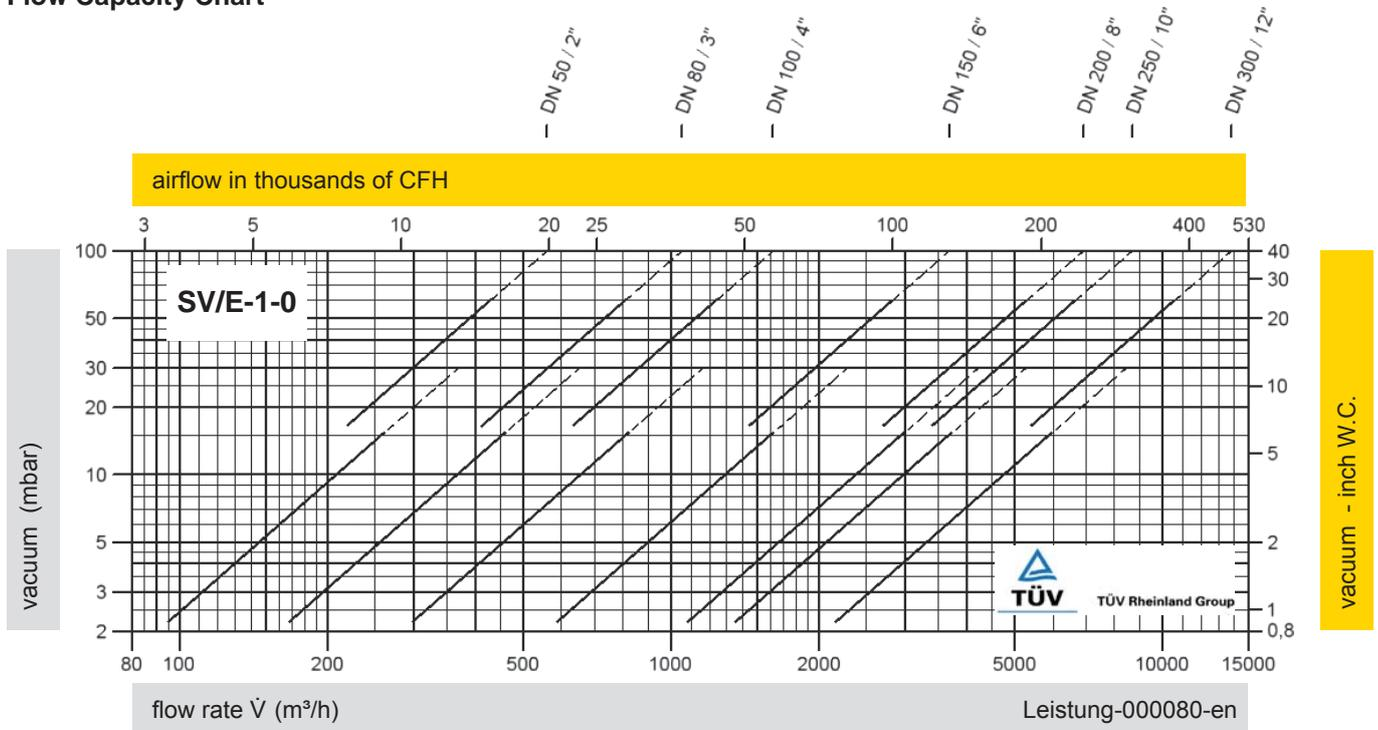
The flow capacity chart has been determined with a calibrated and TÜV certified flow capacity test rig.
