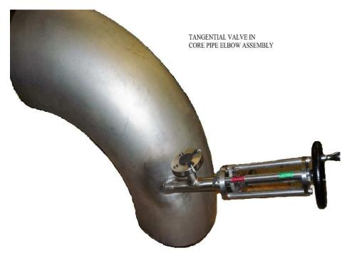
Core pipe assemblies allow close mounting of the valve to the core to eliminate flanges, dead spots and heat losses. The valves can be welded to the core in parallel to the flow, perpendicular to the flow or tangent to the flow depending on the desired effect.
