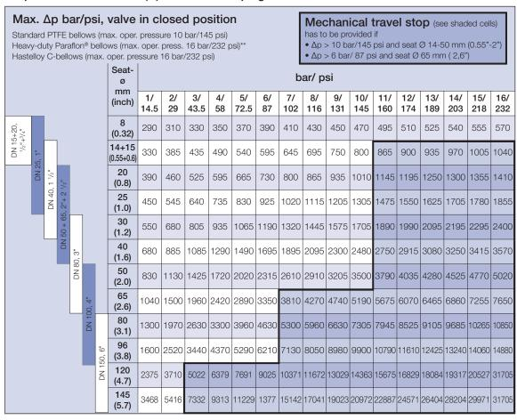
**Attention:** If  $\Delta p < p_2$ , then insert  $p_2$  instead of  $\Delta p$  (see operating limits in pressure/ temperature diagram).
