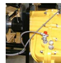
Teflon tubing stainless steel braided with stainless steel fittings and bleed valves
